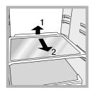
**SHELVES**: with or without grill. Due to the special guides the shelves are removable and the height is adjustable (*see diagram*), allowing easy storage of large containers and food. Height can be adjusted without complete removal of the shelf.
